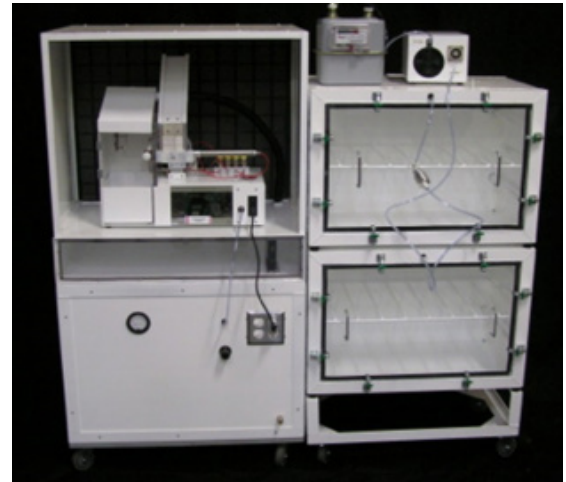
TE-10B US System with mouse chambers & TSP (total suspended particulate) Measuring System
